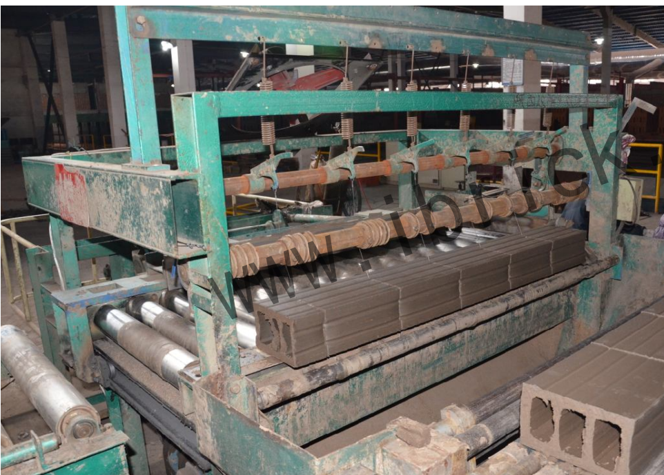
Cut the brick columns into pieces
